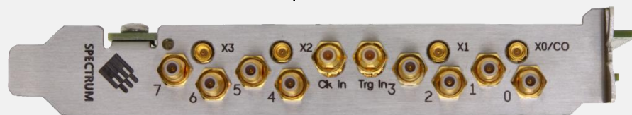
Figure 4: Shows the front panel of an 8-channel card with SMB type connectors for the analogue channels, external clock, and trigger, as well as 4 MMCX connectors for the multipurpose lines.
