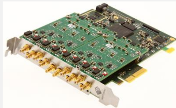
Figure 1: The M2p.5968-x4 Digitizer is a half-size PCIe card with 8 channels all suited to acquiring analogue signals with frequency content up to 60 MHz.
