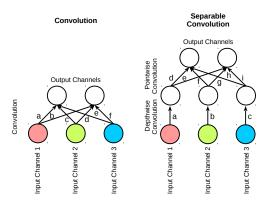
Fig. 1: Comparison of a standard convolution to a separable convolution. The separable convolution first applies a spatial convolution for each channel separately. Afterwards, a convolution with a  $1 \times 1$  kernel is applied. Circles represent one channel of the feature map in the network, arrows a spatial convolution.
