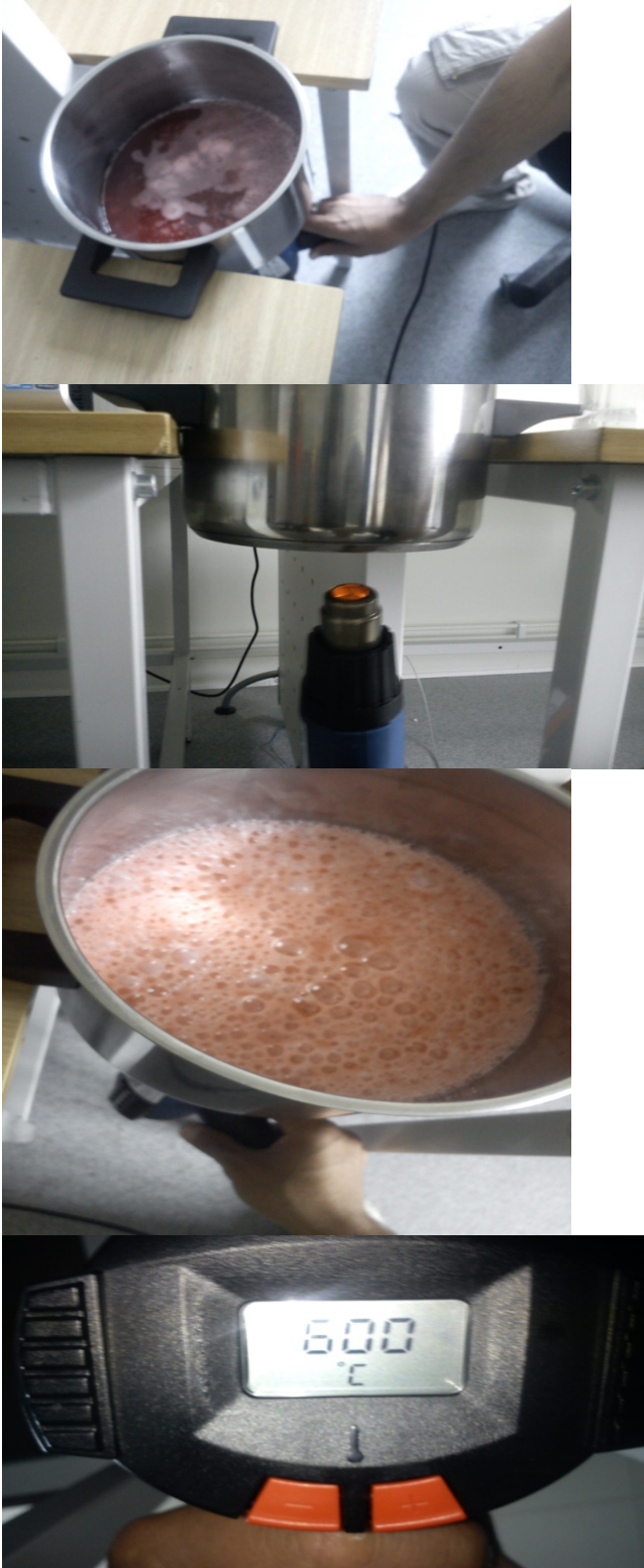
Fig (5.1.3): The operation of heating the mineral oil about 60 minute with a 600 degrees heat source. Figures of artificial aging in the lab.
