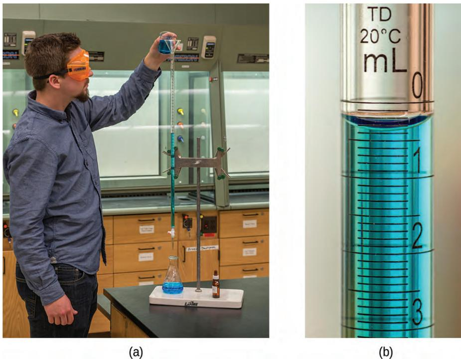
**Figure 4.15** (a) A student fills a buret in preparation for a titration analysis. (b) A typical buret permits volume measurements to the nearest 0.01 mL. (credit a: modification of work by Mark Blaser and Matt Evans; credit b: modification of work by Mark Blaser and Matt Evans)
