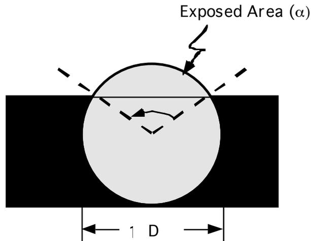
**Figure 6-12. Exposed surface and diameter of trackball.**
