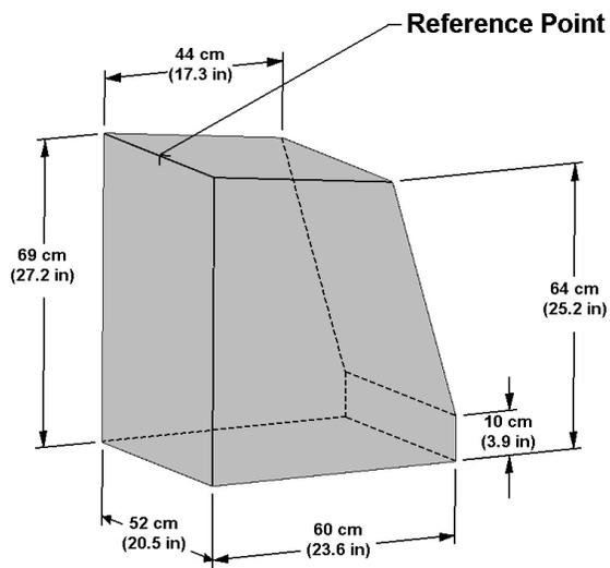
Figure 8.3b Illustration of the Clearance Spaces Used in Method 2 (8.3.2.1.2)
