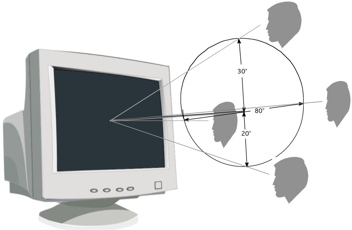
**Figure 7-1. Design angular viewing envelope. When the display surface is viewed from locations outside the design angular viewing envelope, some requirements of the standard, such as contrast luminance, color, contrast, or character size, might not be met (not to scale).**
