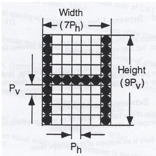
**Figure 7-4. Height and width of characters. The height and width of characters are defined by these figure[EQ: “figure” means grids or pixels?]. Squares represent pixels.  $P_v$  and  $P_h$  represent the vertical and horizontal dimensions of a pixel, respectively.**
