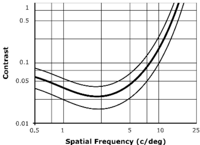
**Figure 7-3. Maximum contrast of moiré patterns. C/deg = cycles per degree of visual angle, and contrast =  $(L_{\max} - L_{\min}) / (L_{\max} + L_{\min})$ , where  $L_{\max}$  is the maximum luminance of the Moiré pattern, and  $L_{\min}$  is its minimum luminance.**
