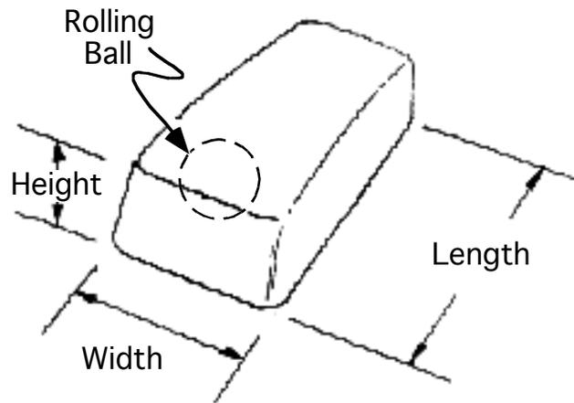
**Figure 6-9. Illustration of a mouse. Note. Many mice use an optical motion sensor rather than a ball.**
