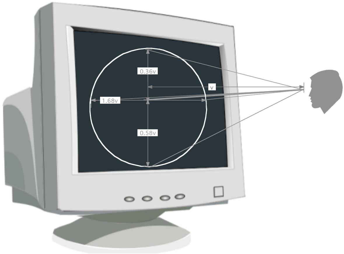
**Figure 7-2. Spatial limits on the display surface imposed by the design angular viewing envelope at the design viewing distance ( $v$ ). Areas of the display surface outside the boundary shown here might not conform to all the requirements of the standard, such as luminance, color, contrast, or character size. This nonconformance occurs when the viewing angle exceeds the angles defined by the design viewing angle envelope (not to scale).**
