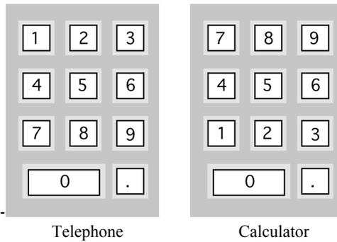
**Figure 6-2. Numeric keypad layouts**
