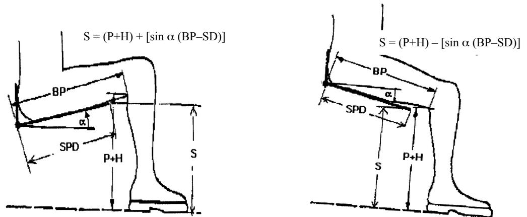
**Figure A-2. Seat height dimensions.** A = abdominal extension depth; H = heel height; S = seat height;  $\alpha$  = seat pan angle; K = knee height, sitting; SPD = seat pan depth; BK = buttock-knee length; P = popliteal height; BP = buttock-popliteal length; T = thigh clearance, sitting; C = clearance.
