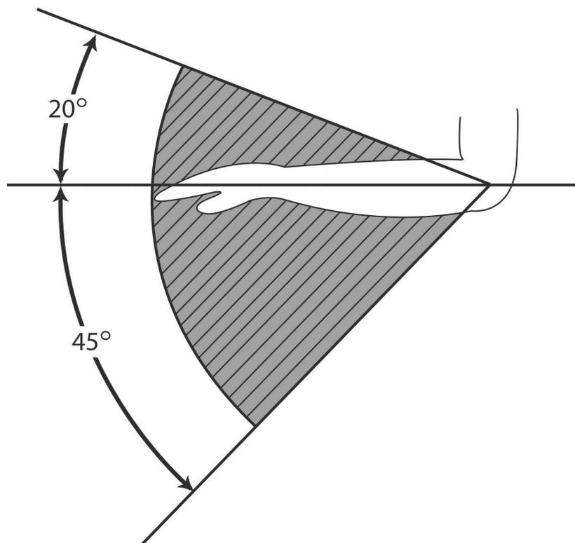
Figure 5-7a. Side view of recommended space (shaded area) for placement of input devices
