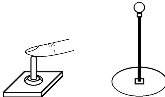
**Figure 6-13. Finger-operated (left) and hand-operated (right) joysticks.**
