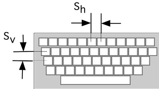
Figure 6-7. Illustration of key spacing.
