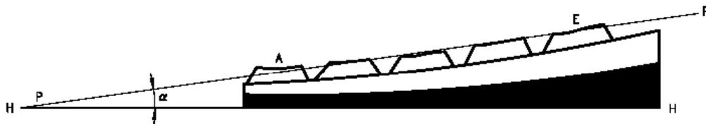
**Figure 6-4. Illustration of keyboard slope. The slope is positive when the A row is lower than the D or E row, and negative when the A row is higher than the D or E row. After ISO 9241, part 4 (ISO, 1998).**
