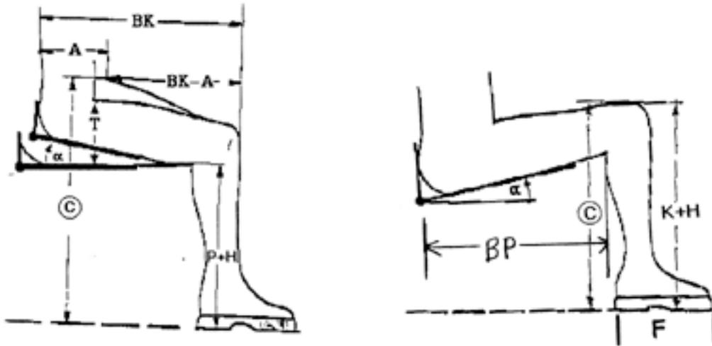
**Figure A-1. Clearance dimensions.** A = abdominal extension depth; H = heel height; F = foot length;  $\alpha$  = seat pan angle; K = knee height, sitting; SPD = seat pan depth; BP = buttock-popliteal length; BK = buttock-knee length; P = popliteal height; T = thigh clearance, sitting; C = clearance.
