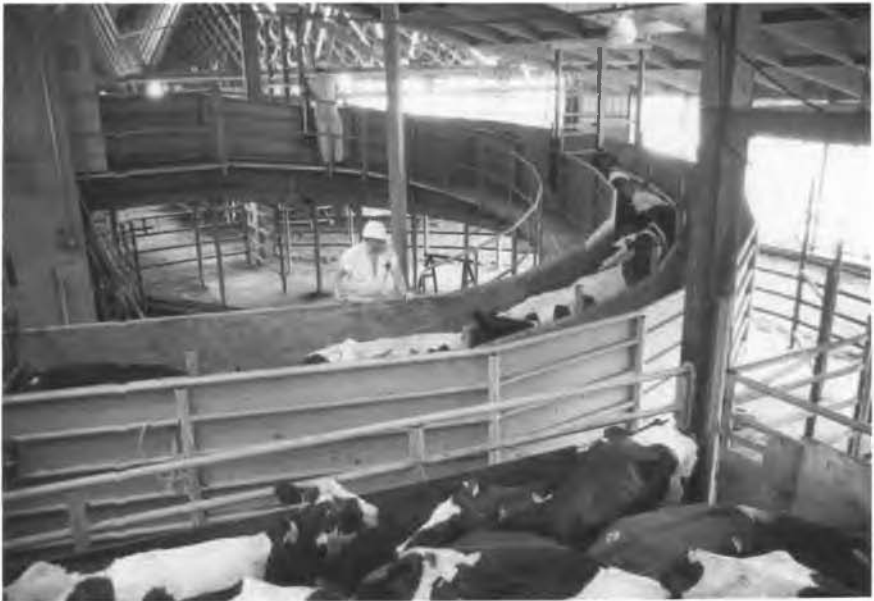
A curved chute with high solid sides utilizes behavior principles to keep cattle calm at the slaughter plant. Photo by Temple Grandin.
