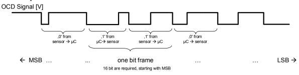
• Typical bit transmission speed (PWM) is:  $\sim$ 0.4  $\mu$ s /  $\sim$ 1.6  $\mu$ s, check after  $\sim$ 1.1  $\mu$ s, wait  $\sim$ 0.4  $\mu$ s (gives  $\sim$ 285 kBit/s).
