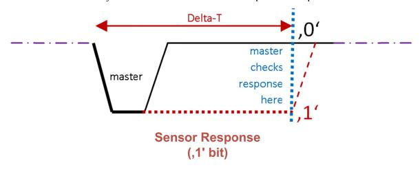
The figure below shows a transmission through the OCD pin as could be seen using an oscilloscope:
