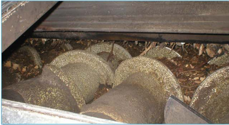
Metering bins equipped with rugged screws improve efficiency and feed biomass in a uniform manner.
