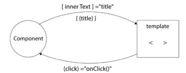
Figure 4.3: Component-template interaction
