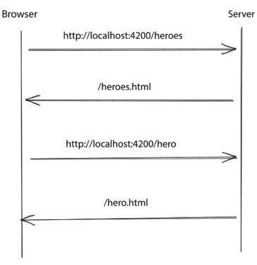
Figure 9.1: Routing in traditional web applications
