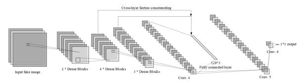
Figure 2. The structure of the proposed common fake feature network.
