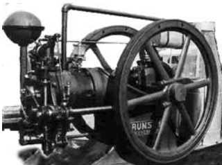
Figure AI8 A Rumsey engine. Note the concentration of mass at the outer periphery of the flywheel
