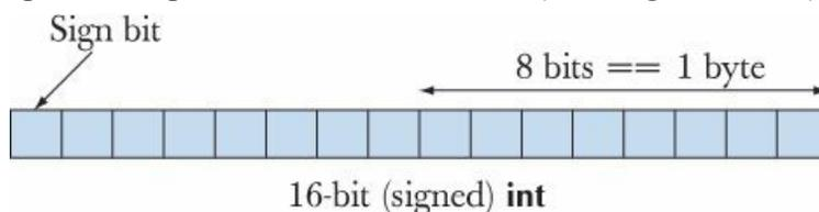
If the sign bit is 1, the number is negative. Almost universally, the two's complement representation is used. To save paper, we consider how we would represent signed numbers in a 4-bit integer:
