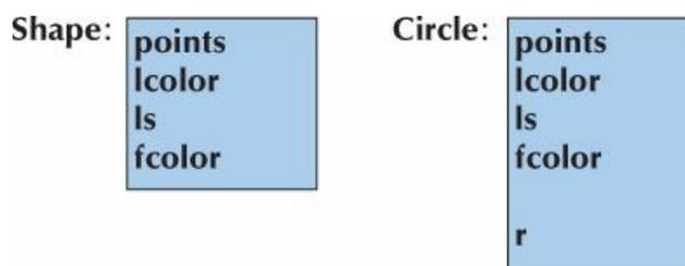
A **Circle** has the data members of a **Shape** (after all, it is a kind of **Shape**) and can be used as a **Shape**. In addition, **Circle** has “its own” data member **r** placed after the inherited data members.
