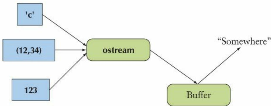
The buffer is a data structure that the **ostream** uses internally to store the data you give it while communicating with the operating system. If you notice a “delay” between your writing to an **ostream** and the characters appearing at their destination, it’s usually because they are still in the buffer. Buffering is important for performance, and performance is important if you deal with large amounts of data.
