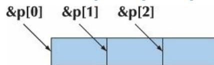
In terms of memory addresses, these pointers are `sizeof(Shape)` apart (§17.3.1). Unfortunately for `poor()`’s caller, `sizeof(Circle)` is larger than `sizeof(Shape)`, so that the memory layout can be visualized like this:
