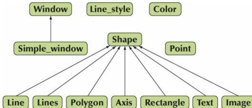
An arrow indicates that the class pointing can be used where the class pointed to is required. For example, a **Polygon** can be used where a **Shape** is required; that is, a **Polygon** is a kind of **Shape**.
