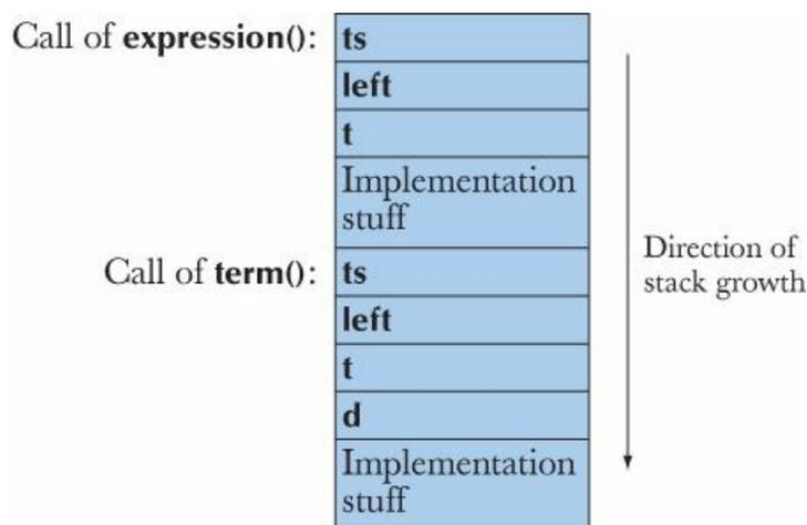
Note that `term()` has an extra variable `d` that needs to be stored, so we set aside space for that in the call even though the code may never get around to using it. That's OK. For reasonable functions (such as every function we directly or indirectly use in this book), the run-time cost of laying down a function activation record doesn't depend on how big it is. The local variable `d` will be initialized only if we execute its `case '/'`.
