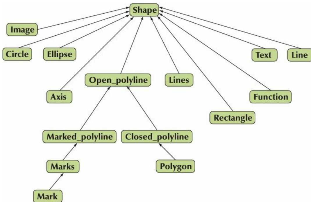
The arrows point from a derived class to its base. Such diagrams help visualize class relationships and often decorate the blackboards of programmers. Compared to commercial frameworks this is a tiny “class hierarchy” with only 16 classes, and only in the case of **Open\_polyline**’s many descendants is the hierarchy more than one deep. Clearly the common base (**Shape**) is the most important class here, even though it represents an abstract concept so that we never directly make a shape.
