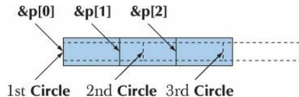
That is, `poor()` is calling `draw()` with a pointer into the middle of the `Circles`! This is likely to lead to immediate disaster (crash).
