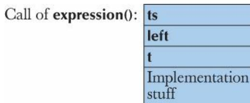
The "implementation stuff" varies from implementation to implementation, but that's basically the information that the function needs to return to its caller and to return a value to its caller. Such a data structure is called a *function activation record*, and each function has its own detailed layout of its activation record. Note that from the implementation's point of view, a parameter is just another local variable.
