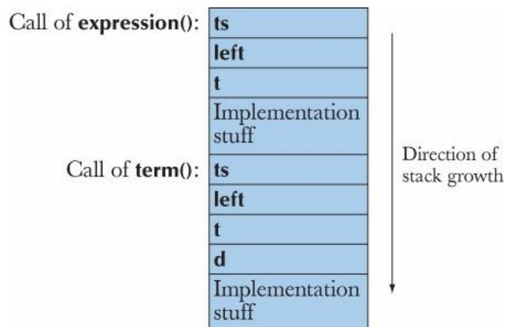
And so on. The stack, also called the *call stack*, is a data structure that grows and shrinks at one end according to the rule “Last in, first out.”
