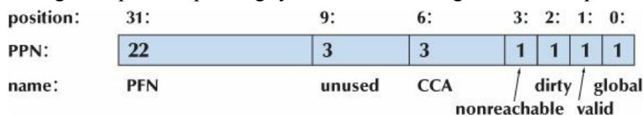
The 32-bit word is used as two numeric fields (one of 22 bits and one of 3 bits) and four flags (1 bit each). The sizes and positions of these pieces of data are fixed. There is even an unused (and unnamed) “field” in the middle. We can express this as a `struct`:
