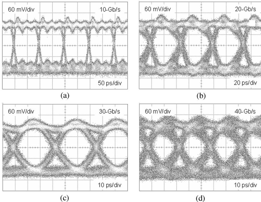
Fig. 16. Measured eye diagram with a  $2^{31}-1$  PRBS input current of  $740 \mu\text{A}_{pp}$  at (a) 10 Gb/s, (b) 20 Gb/s, (c) 30 Gb/s, and (d) 40 Gb/s.
