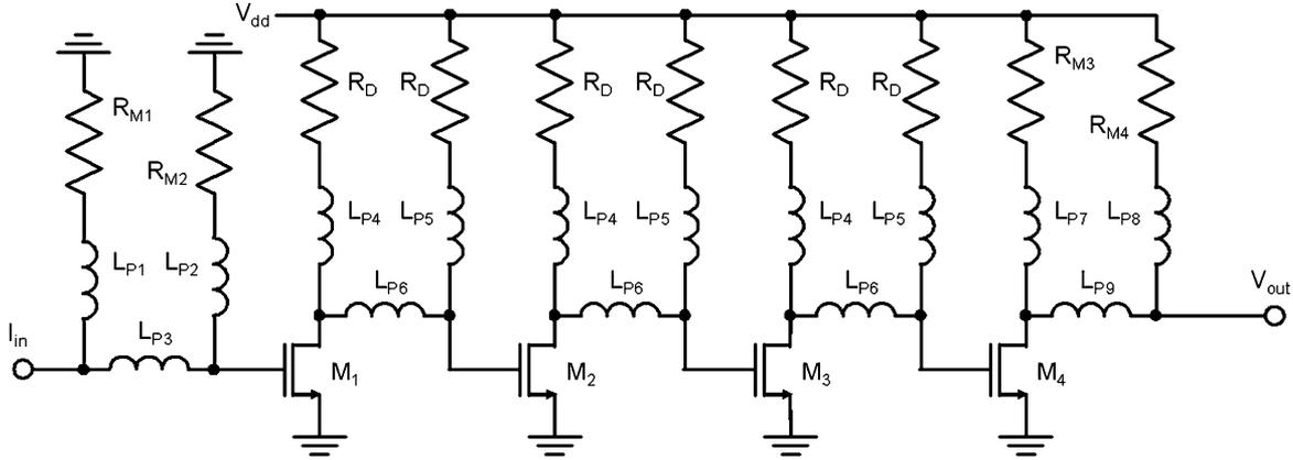
Fig. 7. Circuit topology of the proposed 40-Gb/s CMOS TIA with PIP.
