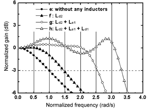
Fig. 4. Comparison of the bandwidth enhancement results using PIP technique under different numbers of peaking inductors, where  $C_g = 3C_d$  and  $R_{d1} = R_{d2}$ .
