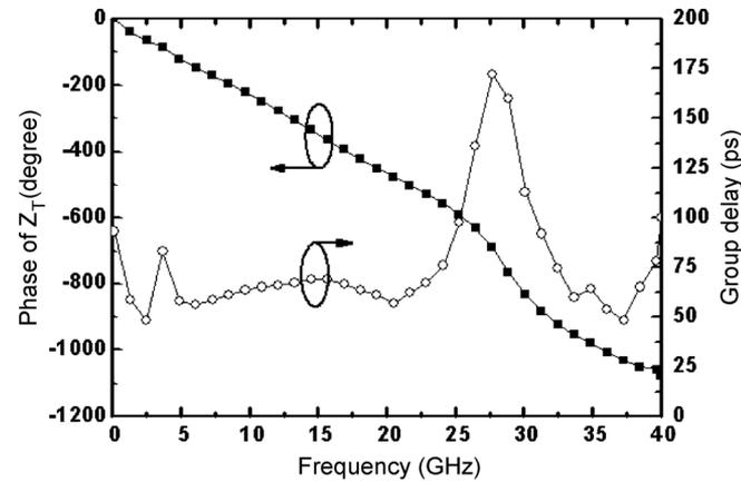
Fig. 13. Measured phase and group delay.
