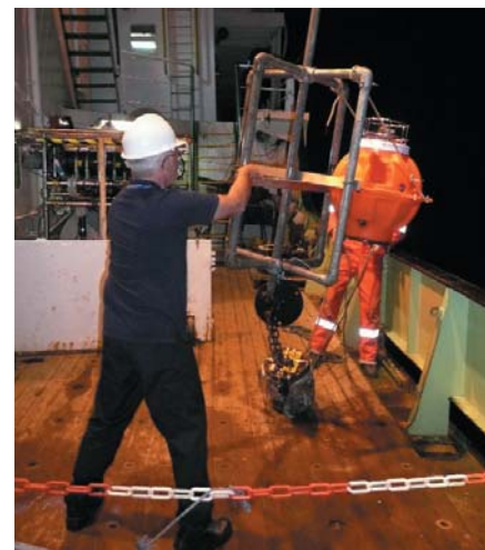
(Above) Fetch is packaged in a spherical pressure housing made from highly pressure tolerant and corrosion-proof glass. It has sufficient battery endurance for deployments of up to five years. (Below) Recent science cruises provided NOC scientists with their first opportunity to carry out tests on Fetch.
