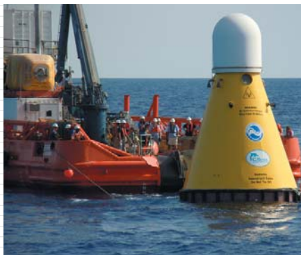
An OceanNet buoy moored some 80km off the southern coast of Cyprus. The buoy is one element of the Offshore Communications Backbone (OCB).
