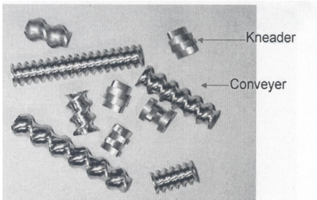
Figure 3. Screw and kneading elements
