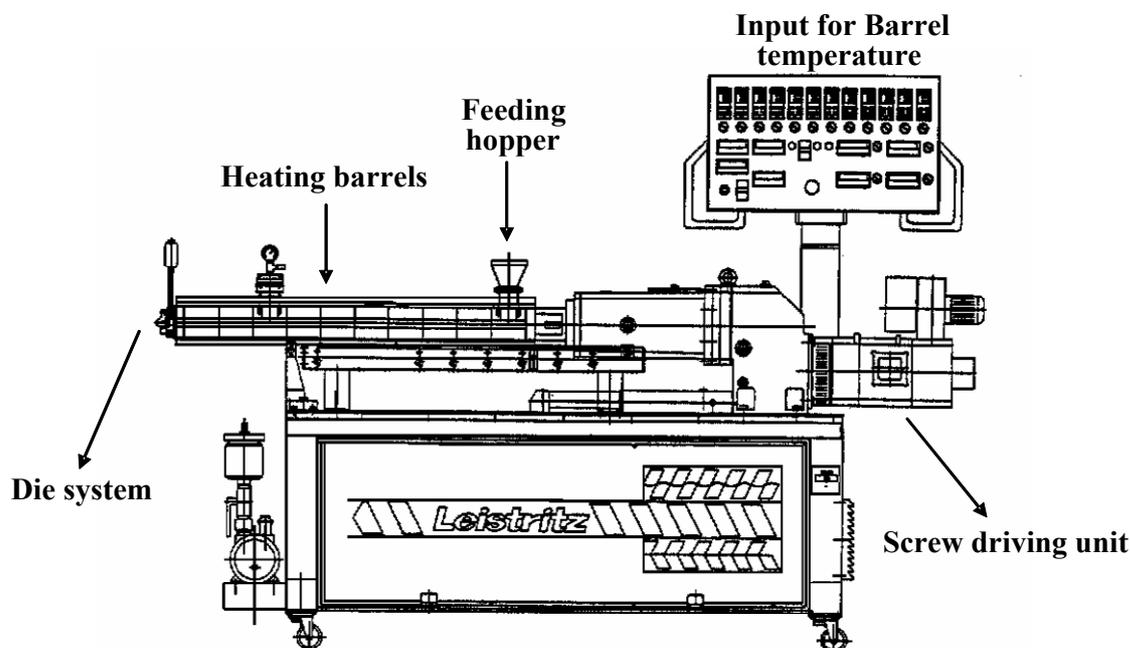
Figure 1. Micro-18 Twin screw co-rotating Leistritz extruder
