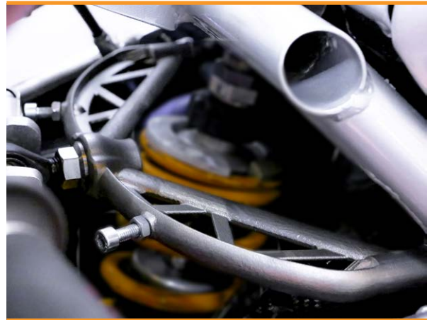
Metal 3D printed one part titanium component on the TransFIORmers bike
