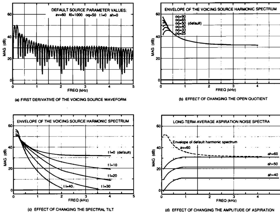
FIG. 11. Dft magnitude spectra are shown of  $U'_g(t)$  ( $U_g(t)$  modified by a first difference approximation to the radiation characteristic), as synthesized by the KLGLOTT88 voicing source model at several values for each of three control parameters. (a) Spectrum of a train of pulses with  $f_0 = 100$  Hz; (b) and (c) spectral envelope of a harmonic spectrum that would result from synthesizing a train of such pulses; (d) spectra of aspiration noise source.
