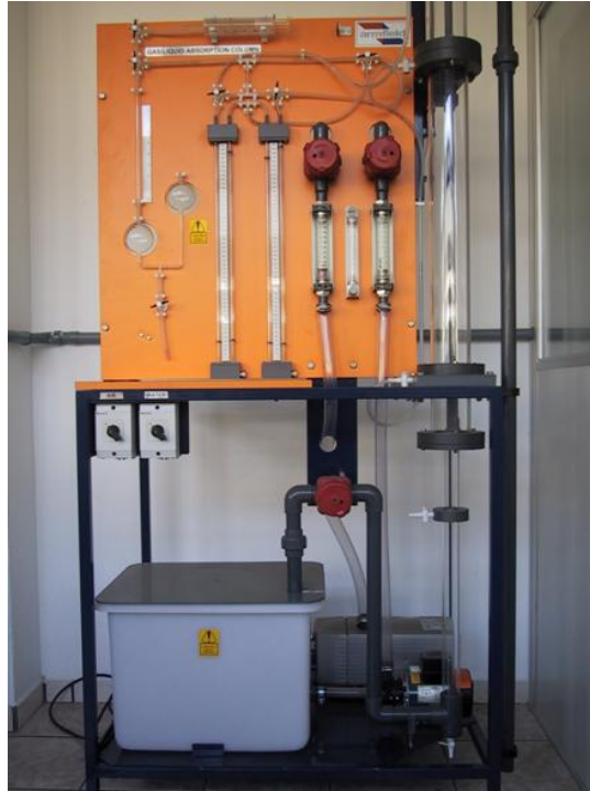
Figure 2 – Gas absorption column.
