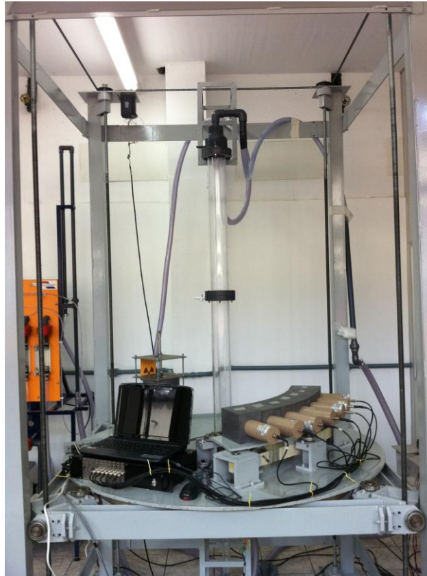
Figure 3. Picture of the third generation CT with the column installed.
