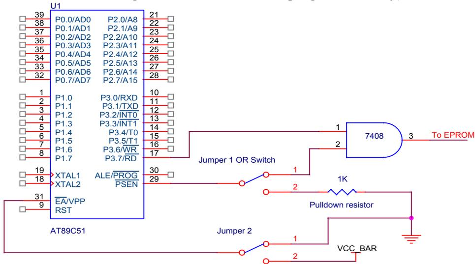
**B) FLIP PROGRAMMING MODE: Both the jumpers are in position 2 at falling edge of reset. /PSEN is then released after reset, so that it can operate normally. Use 1K current limiting resistor for /PSEN pull-down.**
