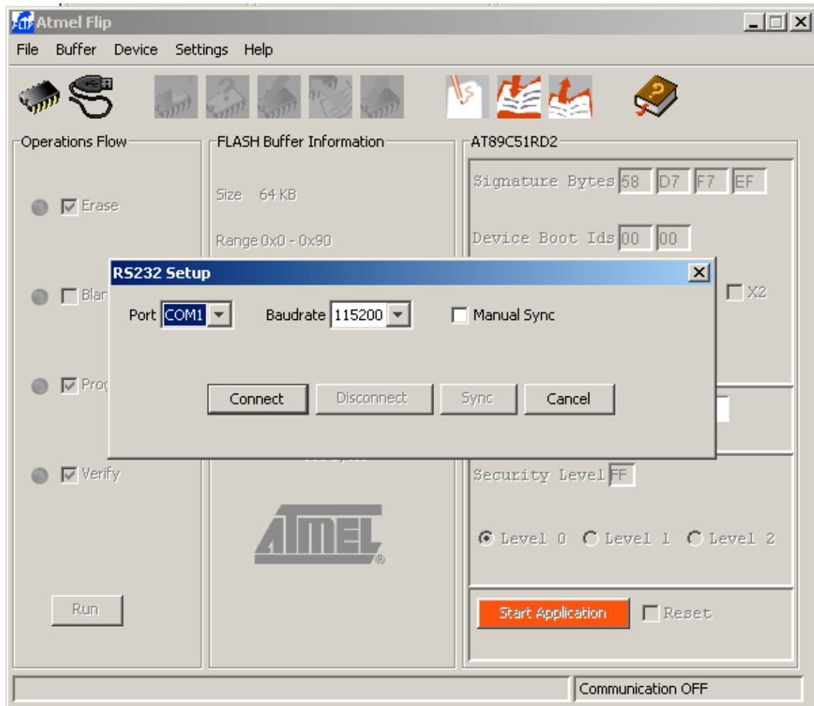
**Step 4:** Load hex file. On loading, the hex file name will be displayed in the center under flash buffer information along with size of it. Then, perform Erase, Blank Check, Program and Verify cycles.
