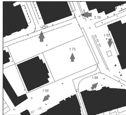
Fig. 5 example of map derived from measurements: average wind speed/ wind direction, summer, 15.00 hrs, Grote Markt, Groningen
