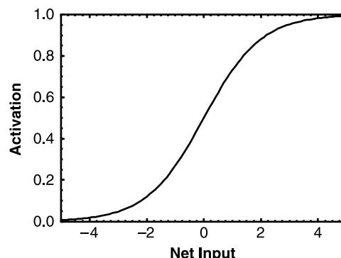
**Figure 2** Nonlinear activation function often used in neural network simulations. The actual function shown, called the logistic function,  $a_i = \frac{1}{1 + e^{-net_i}}$ , is the function most frequently used.
