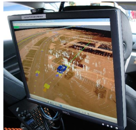
FIGURE 1 [1] A map in a self-driving car that was constructed from sensors gathering information
