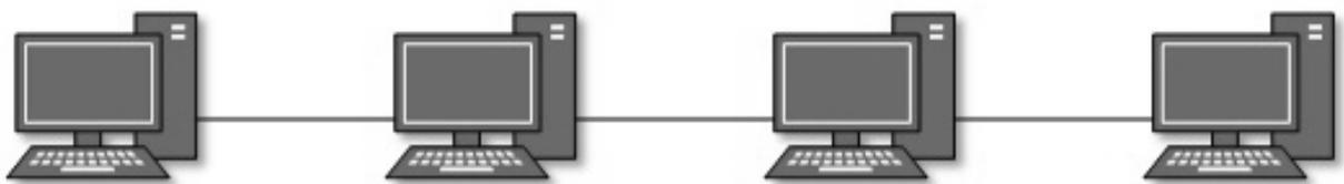
Each link in daisy chain topology represents single point of failure. Every link failure splits the network into two segments. Every intermediate host works as relay for its immediate hosts.
