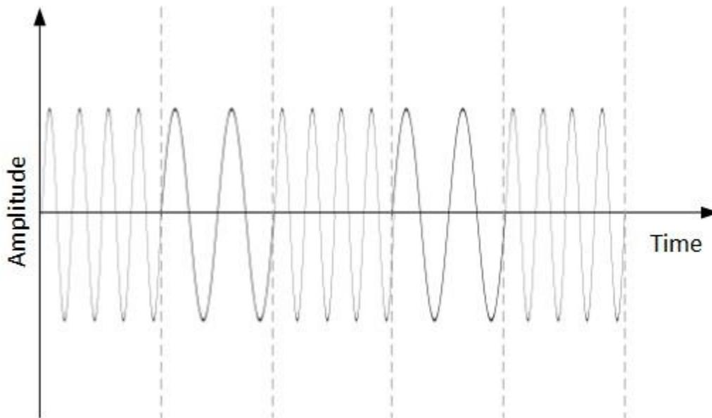
This technique uses two frequencies,  $f_1$  and  $f_2$ . One of them, for example  $f_1$ , is chosen to represent binary digit 1 and the other one is used to represent binary digit 0. Both amplitude and phase of the carrier wave are kept intact.
