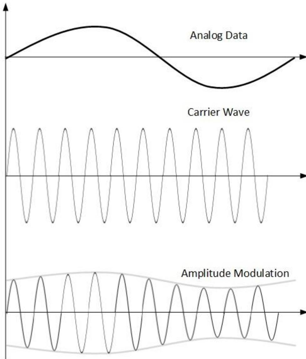
Amplitude modulation is implemented by means of a multiplier. The amplitude of modulating signal (analog data) is multiplied by the amplitude of carrier frequency, which then reflects analog data.
