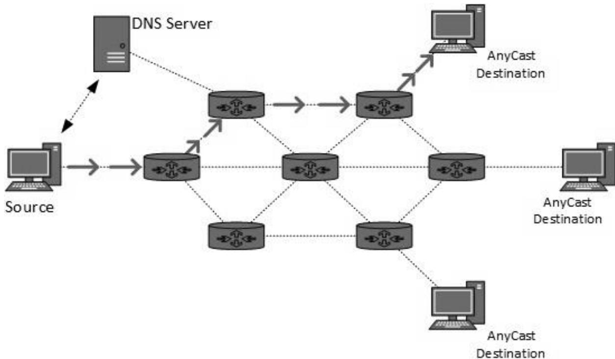
Anycast routing is done with help of DNS server. Whenever an Anycast packet is received it is enquired with DNS to where to send it. DNS provides the IP address which is the nearest IP configured on it.
