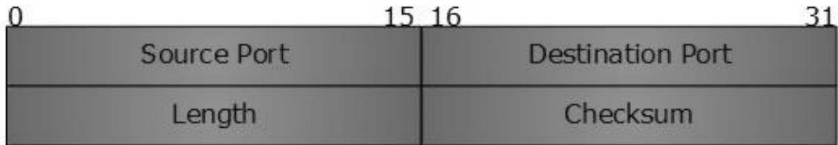
UDP header contains four main parameters:
