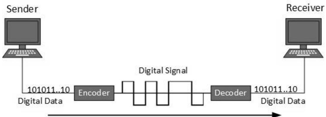
Digital signal is denoted by discrete signal, which represents digital data. There are three types of line coding schemes available:
