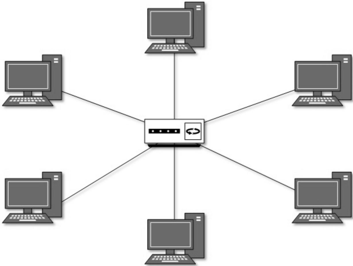
As in Bus topology, hub acts as single point of failure. If hub fails, connectivity of all hosts to all other hosts fails. Every communication between hosts takes place through only the hub. Star topology is not expensive as to connect one more host, only one cable is required and configuration is simple.
