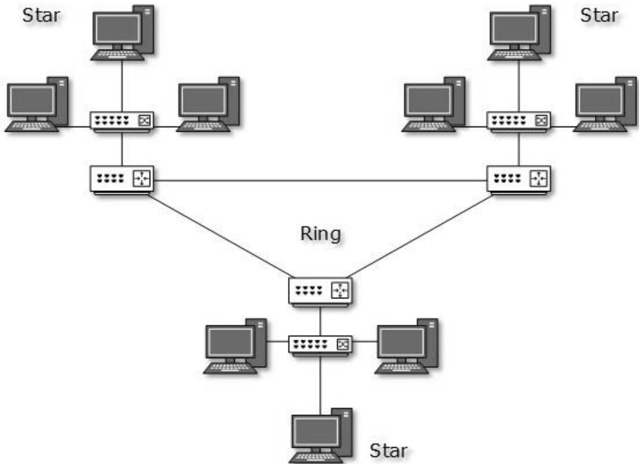
The above picture represents an arbitrarily hybrid topology. The combining topologies may contain attributes of Star, Ring, Bus, and Daisy-chain topologies. Most WANs are connected by means of Dual-Ring topology and networks connected to them are mostly Star topology networks. Internet is the best example of largest Hybrid topology.
