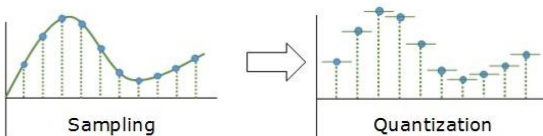
Sampling yields discrete form of continuous analog signal. Every discrete pattern shows the amplitude of the analog signal at that instance. The quantization is done
