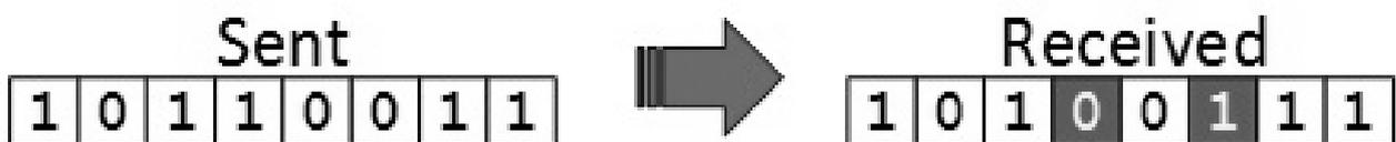
Frame is received with more than one bits in corrupted state.
