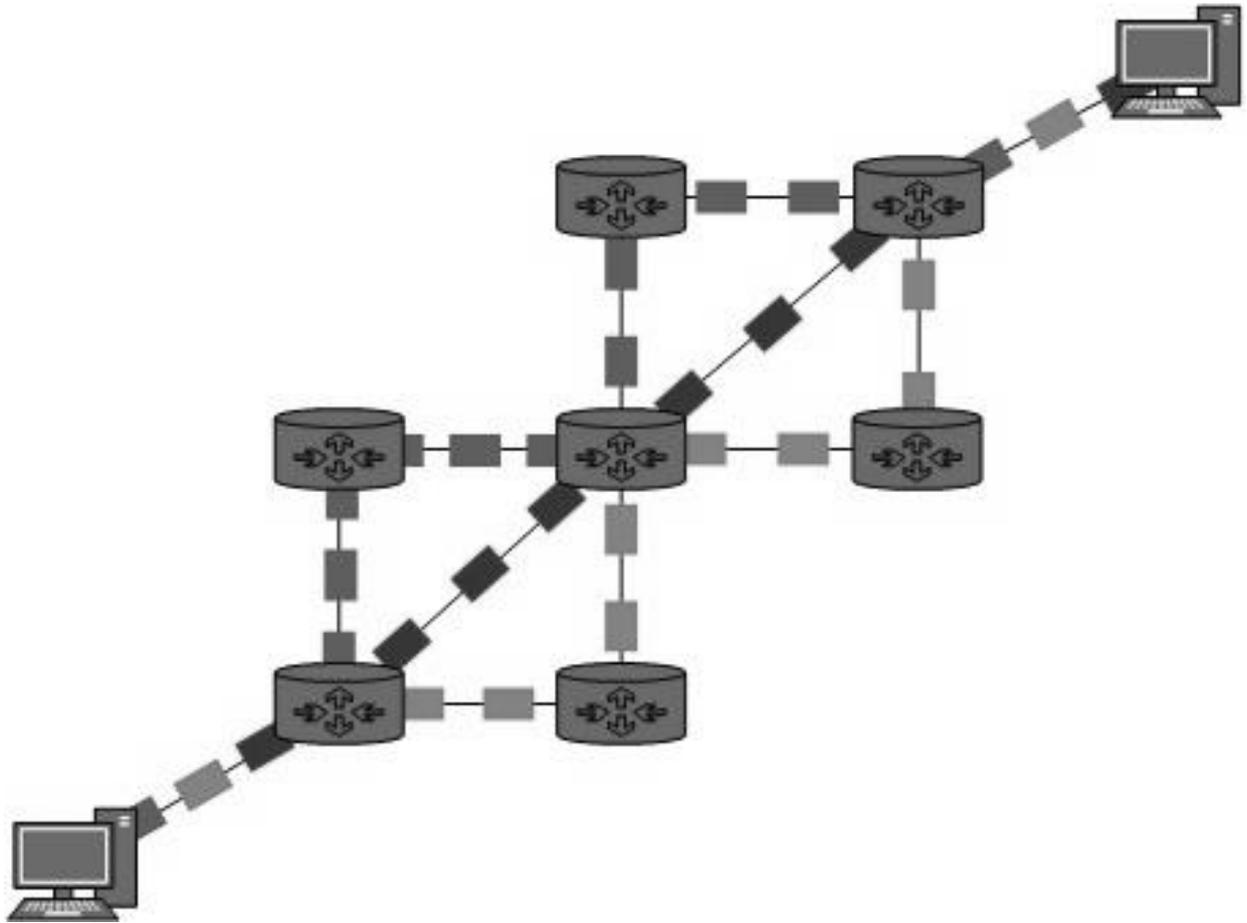
Packet switching enhances line efficiency as packets from multiple applications can be multiplexed over the carrier. The internet uses packet switching technique. Packet switching enables the user to differentiate data streams based on priorities. Packets are stored and forwarded according to their priority to provide quality of service.
