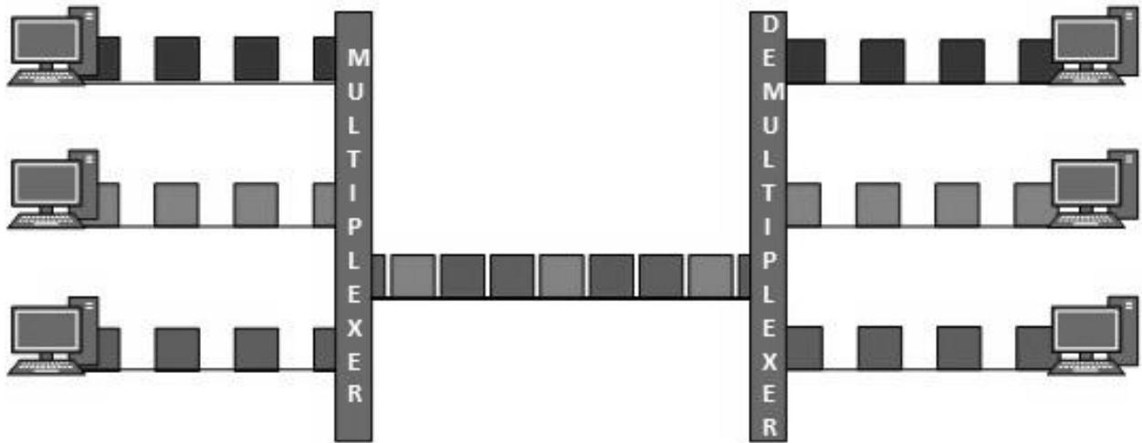
When channel A transmits its frame at one end, the De-multiplexer provides media to channel A on the other end. As soon as the channel A's time slot expires, this side switches to channel B. On the other end, the De-multiplexer works in a synchronized manner and provides media to channel B. Signals from different channels travel the path in interleaved manner.
