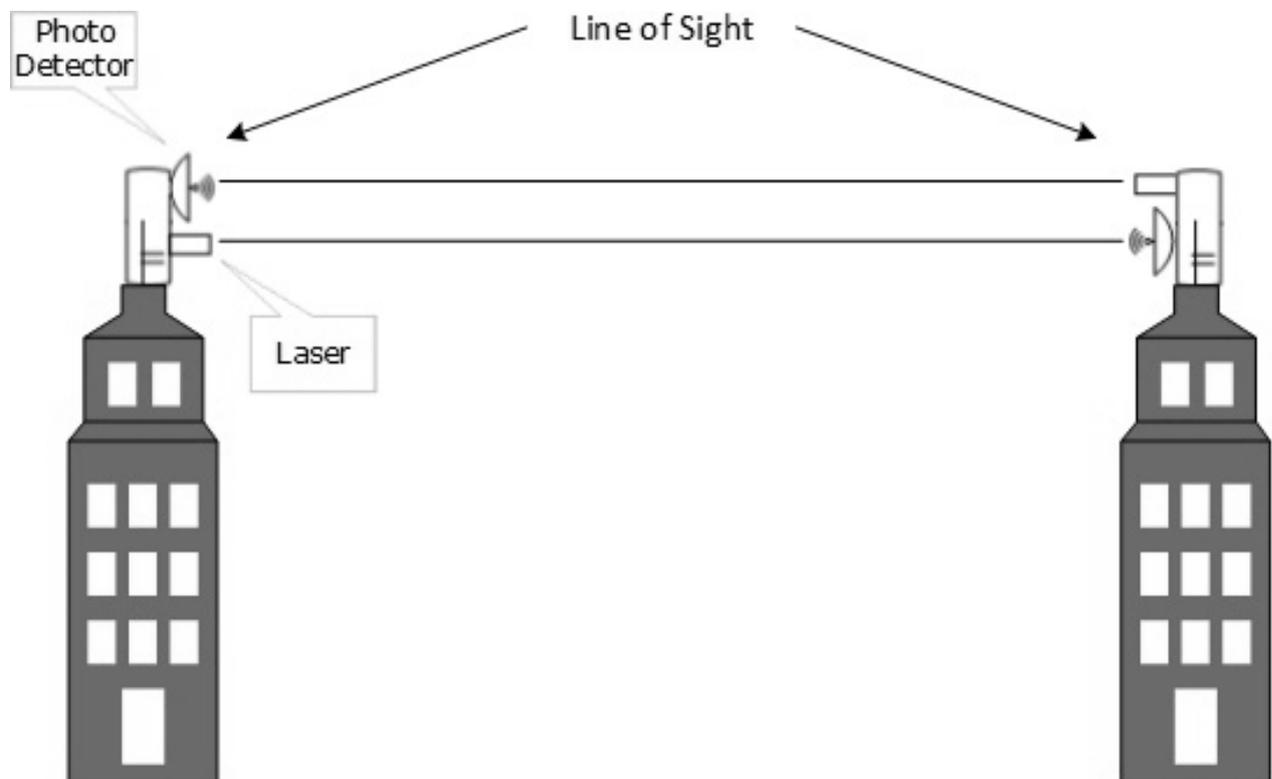
Laser works as Tx (transmitter) and photo-detectors works as Rx (receiver).
