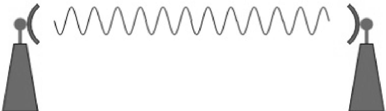
Microwave antennas concentrate the waves making a beam of it. As shown in picture above, multiple antennas can be aligned to reach farther. Microwaves have higher frequencies and do not penetrate wall like obstacles.
