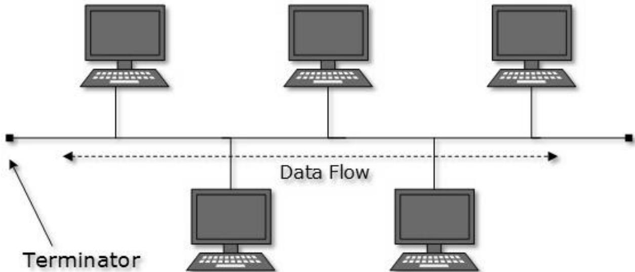
Both ends of the shared channel have line terminator. The data is sent in only one direction and as soon as it reaches the extreme end, the terminator removes the data from the line.
