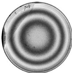
Fig. 3: Example of a GaN-HEMT epitaxial wafer exhibiting quite high surface roughness (rms=9.2 nm) and moderate GaN buffer layer uniformity (thickness standard deviation of 3.2 % and total thickness variation of 9 %) visualized by Candela™ inspection. An extended defect line in the substrate is detected here, too.
