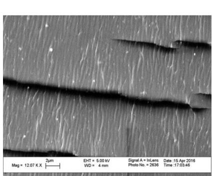
■ NaCl solution in water with UV illumination degraded multilayer stack
