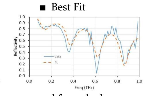
■ Effective refractive index extracted from the best fit:  $\tilde{n} = 1.88 - i6.79 \times 10^{-2}$
