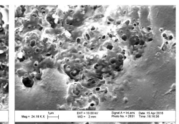
■ Humidity and UV degraded multilayer stack
