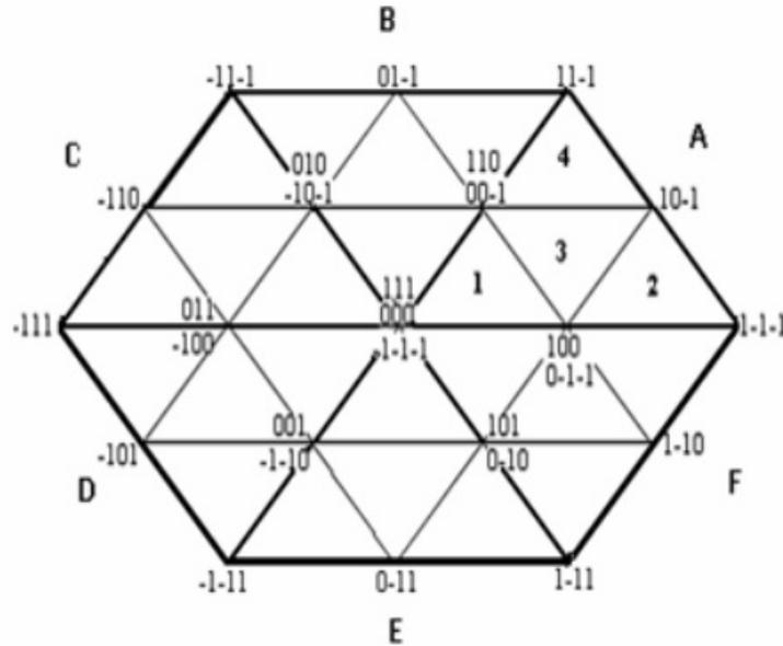
Figure 7: Space Vector Diagram of a Three Level Inverter
