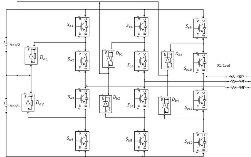
Figure 5: Three Level Diode Clamped Multilevel Inverter
