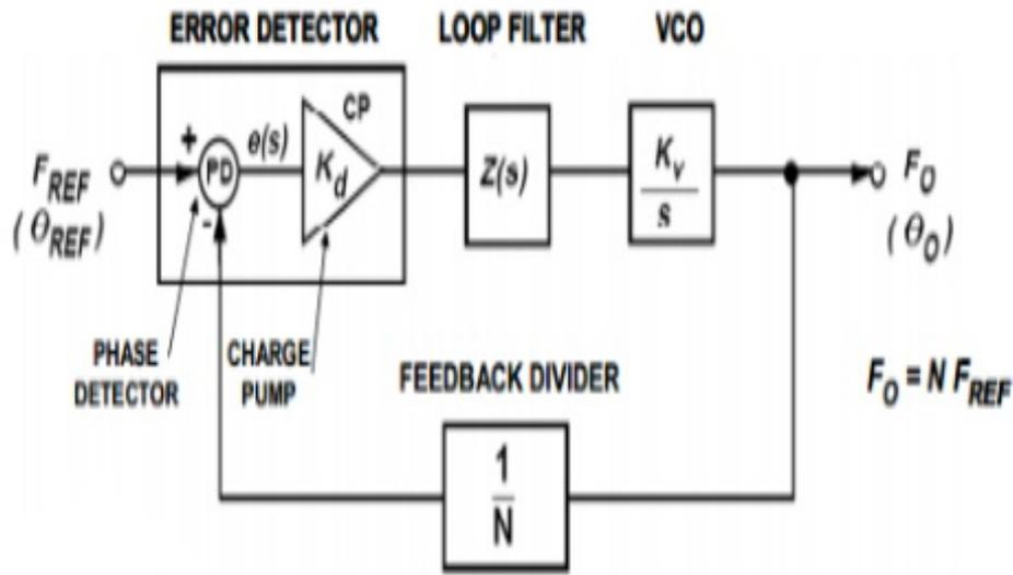
Figure 8: Phase Locked Loop
