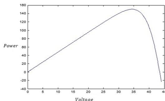
Figure 9: Voltage Power Waveform of PV
