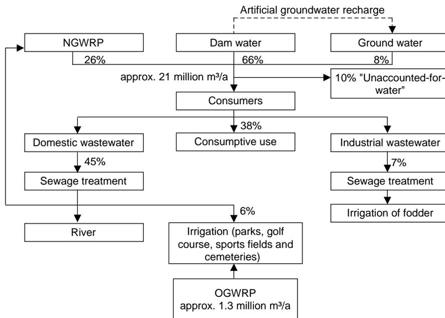
**Figure 1** Water sources and water supply to Windhoek (modified for 2004 after Van der Merwe, 2000)
