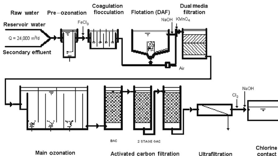
**Figure 2** NGWRP process flow diagram
