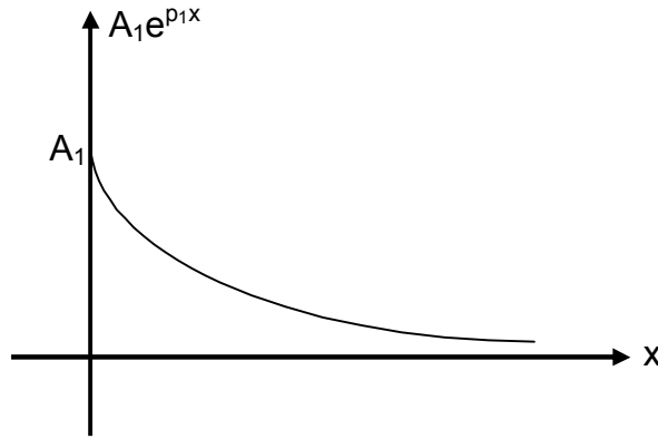
Figure 2.3 A negative real solution generates an unstable orbital motion with decreasing amplitude
