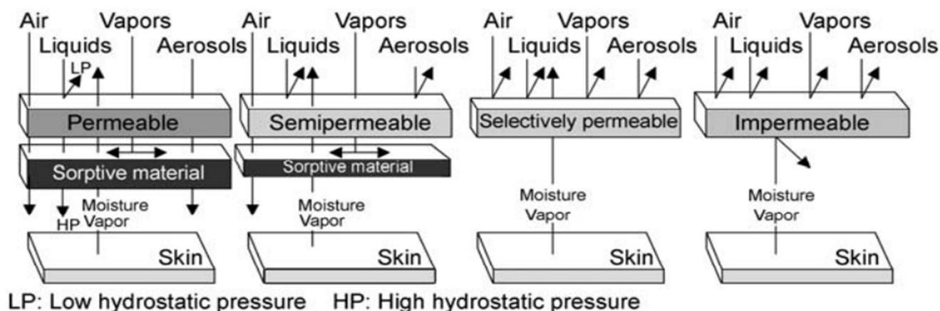
Figure 1. Different types of protective materials.
