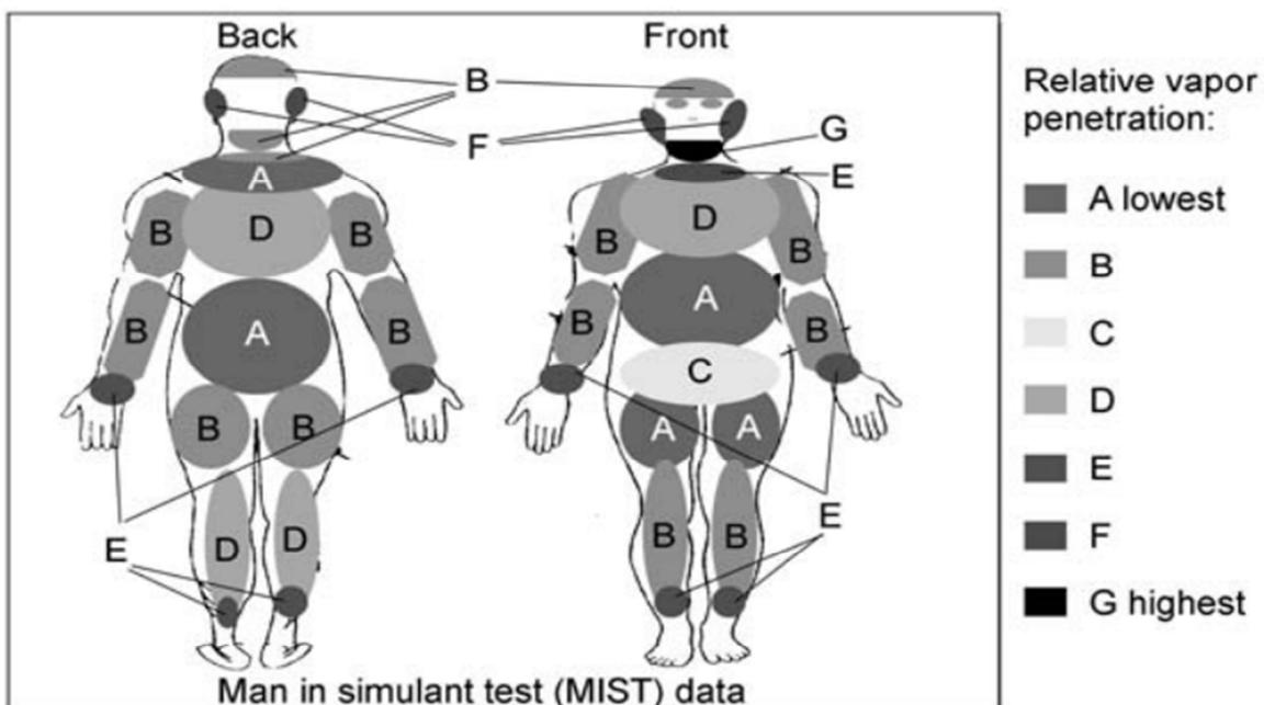
Figure 3. Vapor penetration resistance of a candidate ensemble.
