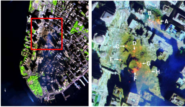
Fig. 6. AVIRIS hyperspectral image collected over the World Trade Center (left) and detail of the area used as input query (right).
