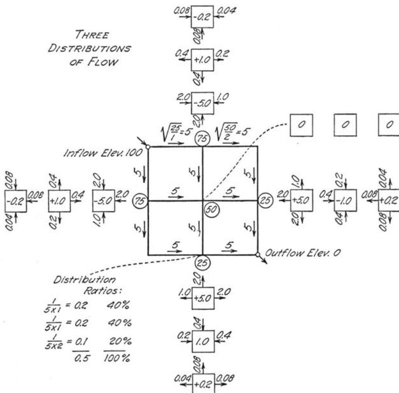
FIG. 6. DISTRIBUTION OF FLOW IN SIMPLE NETWORK; METHOD OF BALANCING FLOWS
