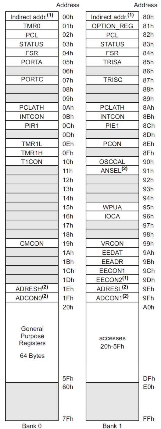
Fig. 3: Address space of a popular microcontroller series (PIC 16F630/16F637). Writing data to addresses between 20h and 5fh stores it in the internal RAM. Writing to other address locations accesses the specified peripheral function.
