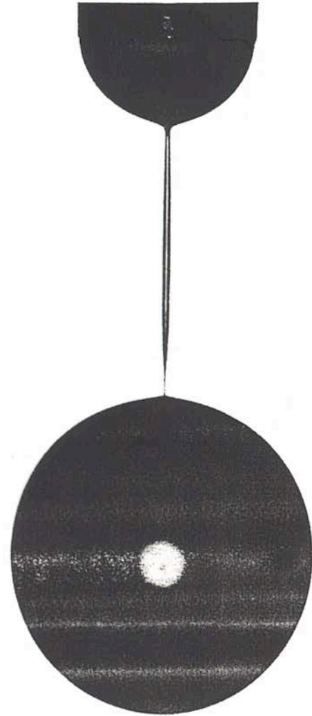
FIG. 7. A drop of a glycerol and water mixture, 100 times as viscous as water, falling from a nozzle 1.5 mm in diameter. As opposed to the case of water, a long neck is produced (Shi, Brenner, and Nagel, 1994). Reprinted with permission. © American Association for the Advancement of Science.
