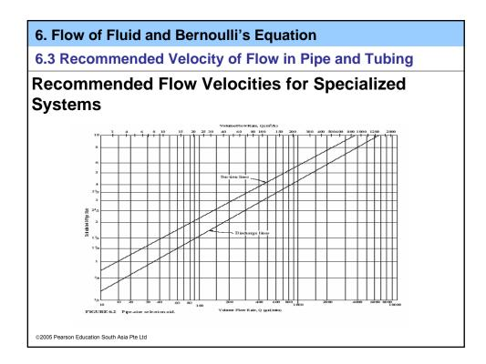
6.3 Recommended Velocity of Flow in Pipe and Tubing
