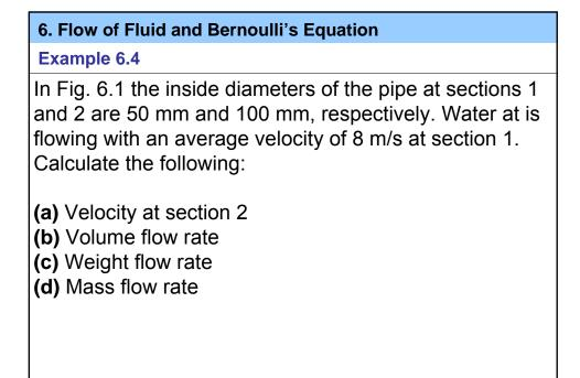
6. Flow of Fluid and Bernoulli's Equation Example 6.4 (a) Velocity at section 2. From Eq. (6–5) we have  $A_1v_1 = A_2v_2$   $v_2 = v_1 \left(\frac{A_1}{A_2}\right)$   $A_1 = \frac{\pi D_1^2}{4} = \frac{\pi (50 \text{ mm})^2}{4} = 1963 \text{ mm}^2$   $A_2 = \frac{\pi D_2^2}{4} = \frac{\pi (100 \text{ mm})^2}{4} = 7854 \text{ mm}^2$
