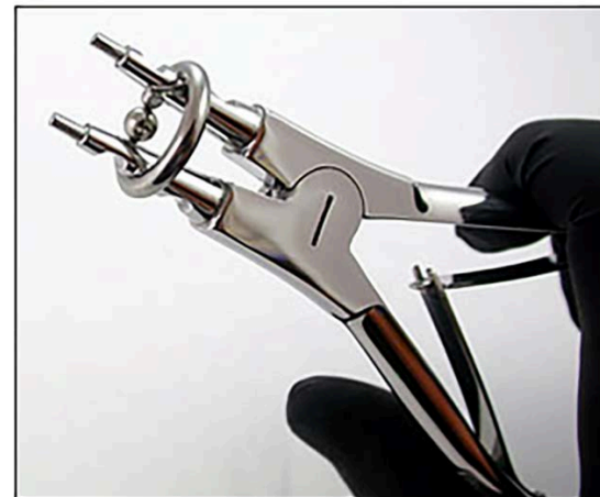
Figure 24. Ring expanding pliers being used to expand ring.
