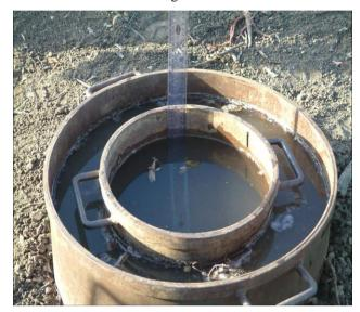
Figure.2. Simple Double Ring Infiltrometer
