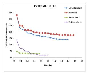
Figure.5 Infiltration capacity curve for Pichinaidupalli village
