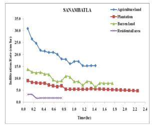
Figure.3 Infiltration capacity curve for sanambatla village
