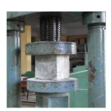
Fig 5: Compressive strength test
