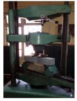
Fig 6: Split tensile strength test
