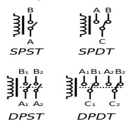
Fig.1 Types of switches
