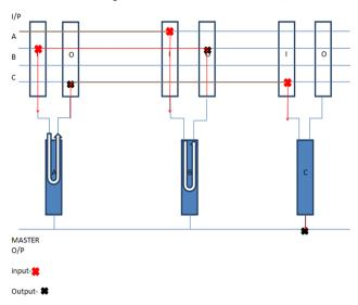
Fig.4 Switching Network using Multiplexer
