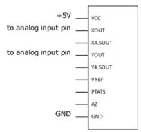
Figure.3.5 pin diagram of gyro
