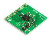
Image.3.2. Gyro breakout board
