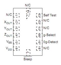
Figure.3.3 pin diagram of accelerometer
