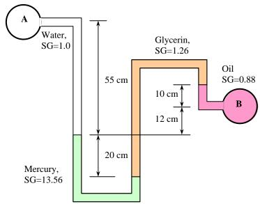
**Discussion** Using a manometer between two pipes is not recommended unless the pressures in the two pipes are relatively constant. Otherwise, an over-rise of pressure in one pipe can push the manometer fluid into the other pipe, creating a short circuit.
