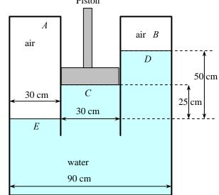
$$P_{\text{air A}} = P_E = P_C + \rho g \overline{CE} = P_{\text{atm}} + \frac{W_{\text{piston}}}{A_{\text{piston}}} + \rho g \overline{CE}$$
