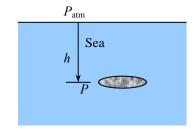
The pressure exerted on the surface of the submarine cruising 300 ft below the free surface of the sea is the absolute pressure at that location:
