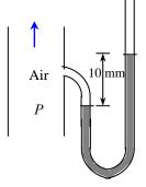
**Discussion** When measuring pressures in a fluid flow, the *difference* between two pressures is usually desired. In this case, the difference is between the measurement point and atmospheric pressure.
