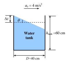
**Assumptions** 1 The road is horizontal during acceleration so that acceleration has no vertical component  $(a_z = 0)$ . 2 Effects of splashing, breaking, driving over bumps, and climbing hills are assumed to be secondary, and are not considered. 3 The acceleration remains constant.
