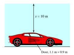
(b) When the car is filled with water, the net force normal to the surface of the door is **zero** since the pressure on both sides of the door will be the same.
