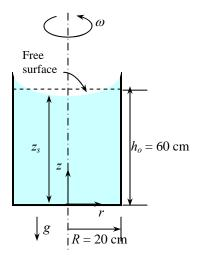
Assumptions 1 The increase in the rotational speed is very slow so that the liquid in the container always acts as a rigid body. 2 The bottom surface of the container remains covered with liquid during rotation (no dry spots).
