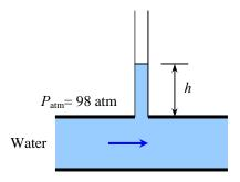
**Discussion** Even though the water is flowing, the water in the tube itself is at rest. If the pressure at the tube bottom had been given in terms of gage pressure, we would not have had to take into account the atmospheric pressure term.
