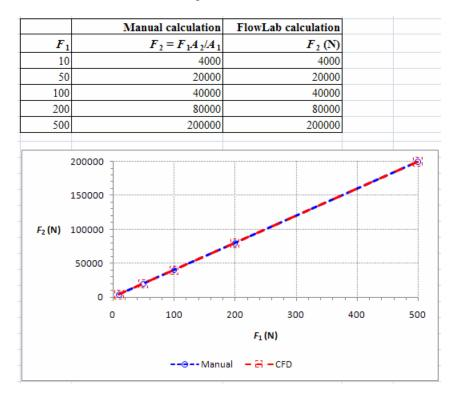
The agreement between the manual and CFD calculations is excellent as expected since this is a simple hydrostatics problem. We also verify on the plot that the relationship between  $F_2$  and  $F_1$  is indeed linear.
