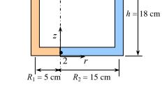
The pressure at point 2 is the same for both fluids, so are the pressures at points 1 and 1\*  $(P_1 = P_1^* = P_{atm})$ . Therefore,  $P_2 - P_1$  is the same for both fluids. Noting that  $z_2 - z_1 = -h$  for both fluids and expressing  $P_2 - P_1$  for each fluid,
