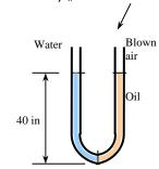
**Discussion** When the person stops blowing, the oil rises and some water flows into the right arm. It can be shown that when the curvature effects of the tube are disregarded, the differential height of water is 23.7 in to balance 30-in of oil.
