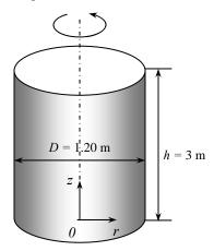
**Assumptions** 1 The increase in the rotational speed is very slow so that the liquid in the container always acts as a rigid body. 2 Gasoline is an incompressible substance.
