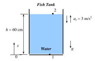
**Assumptions** 1 The acceleration remains constant. 2 Water is an incompressible substance.
