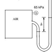
**Discussion** The manometer with water is more precise since the column height is bigger (better resolution). However, a column of water more than 8 meters high would be impractical, so mercury is the better choice of manometer fluid here. *Note*: Mercury vapors are hazardous, and the use of mercury is no longer encouraged.
