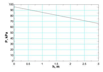
**Discussion** Note that the pressure at the piston face decreases, and the force needed to raise water increases linearly with increasing height of water column relative to the free surface.
