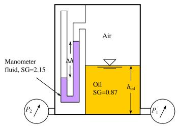
**Discussion** The negative pressure difference indicates that the pressure differential across the oil level is greater than the pressure differential corresponding to the differential height of the manometer fluid.
