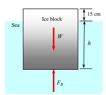
**Solution** If only 10% of an iceberg is above the water surface, the density of the iceberg is to be determined.
