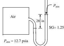
**Solution** The pressure in a pressurized water tank is measured by a multi-fluid manometer. The gage pressure of air in the tank is to be determined.
