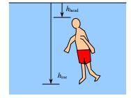
$$P_{\text{toe}} - P_{\text{head}} = \rho g h_{\text{toe}} - \rho g h_{\text{head}} = \rho g (h_{\text{toe}} - h_{\text{head}})$$
