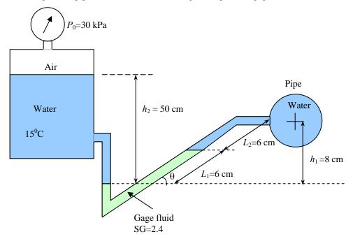
**Discussion** Note that even without a manometer, the reading of a pressure gage can be in error if it is not placed at the same level as the pipe when the fluid is a liquid.
