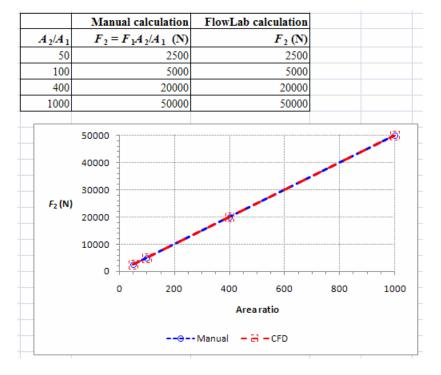
The **agreement between the manual and CFD calculations is excellent** as expected since this is a simple hydrostatics problem. We also verify on the plot that the relationship between  $F_2$  and  $A_2/A_1$  is indeed linear.
