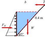
The vertical force on the horizontal surface is zero since it coincides with the free surface of water. The weight of fluid block per 3-m length is
