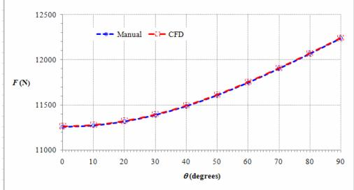
The agreement between the manual and CFD calculations is excellent as expected since this is a simple hydrostatics problem. The percentage difference between the manual and CFD calculations is less than 0.04% for all the cases. We also verify on the plot that the relationship between F and h is indeed **nonlinear**.
