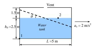
**Assumptions** 1 The road is horizontal during acceleration so that acceleration has no vertical component  $(a_z = 0)$ . 2 Effects of splashing, breaking and driving over bumps are assumed to be secondary, and are not considered. 3 The vent is never blocked, and thus the minimum pressure is the atmospheric pressure.
