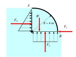
*The weight of fluid block per 4-m length* (downwards):
