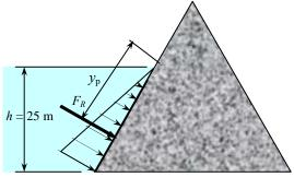
$$\begin{split} F_R &= P_{\text{avg}} A = \left( P_{\text{atm}} + \rho g h_C \right) A \\ &= \left[ 100,000 \text{ N/m}^2 + \left( 1000 \text{ kg/m}^3 \right) \left( 9.81 \text{ m/s}^2 \right) \left( 12.5 \text{ m} \right) \right] \left( 150 \times 28.87 \text{ m}^2 \right) \left( \frac{1 \text{ N}}{1 \text{ kg} \cdot \text{m/s}^2} \right) \\ &= \mathbf{9.64} \times \mathbf{10^8 N} \end{split}$$
