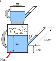
**Discussion** We can obtain the same result formally by starting with the vapor pressure in the teapot and moving along the service tube by adding (as we go down) or subtracting (as we go up) the  $\rho gh$  terms until we reach the atmosphere, and setting the result equal to  $P_{\text{atm}}$ :
