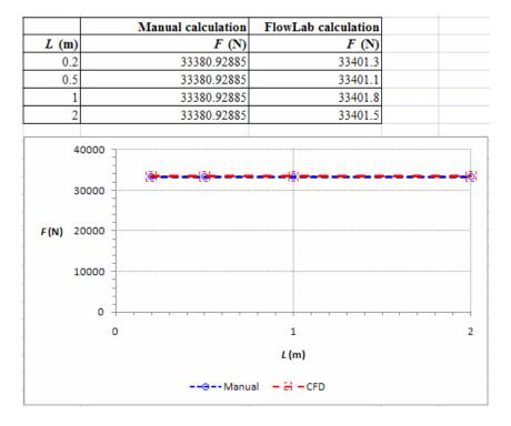
The agreement between the manual and CFD calculations is excellent as expected since this is a simple hydrostatics problem. We also verify on the plot that the F is not a function of L.
