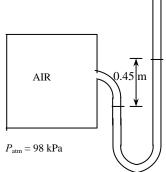
**Discussion** If a heavier liquid, such as water, were used for the manometer fluid, the column height would be smaller, and thus the reading would be less precise (lower resolution).
