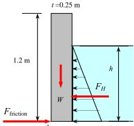
**Solution** A retaining wall against mud slide is to be constructed by rectangular concrete blocks. The mud height at which the blocks will start sliding, and the blocks will tip over are to be determined.
