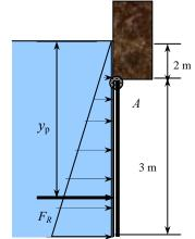
**Discussion** You can calculate the force at point B required to hold back the gate by setting the net moment around hinge point A to zero.
