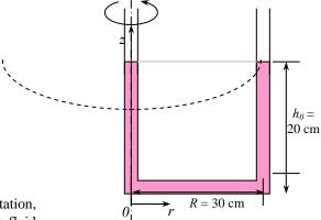
$$\Delta h = z_s(R) - z_s(0) = \left(h_0 + \frac{\omega^2 R^2}{4g}\right) - \left(h_0 - \frac{\omega^2 R^2}{4g}\right) = \frac{\omega^2 R^2}{2g} = \frac{(4.2 \text{ rad/s})^2 (0.30 \text{ m})^2}{2(9.81 \text{ m/s}^2)} = \mathbf{0.081 m}$$
