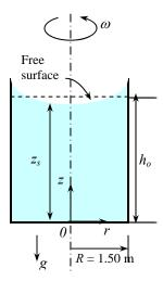
**Assumptions** 1 The increase in the rotational speed is very slow so that the liquid in the container always acts as a rigid body. 2 Milk is an incompressible substance.
