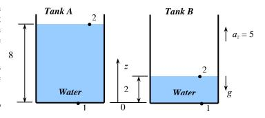
Analysis The pressure difference between two points 1 and 2 in an incompressible fluid is given by
