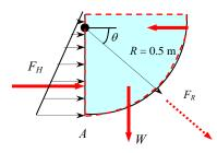
Then the magnitude and direction of the hydrostatic force acting on the surface of the 3-m long section of the trough become
