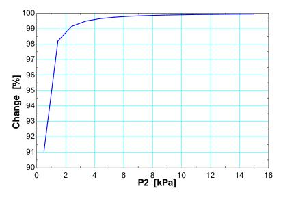
**Discussion** The change in cable tension is at first very rapid, but levels off as the balloon shrinks to nearly zero diameter at high pressure.
