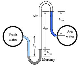
**Solution** Fresh and seawater flowing in parallel horizontal pipelines are connected to each other by a double U-tube manometer. The pressure difference between the two pipelines is to be determined.
