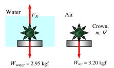
which is considerably less than the density of gold. Therefore, the crown is NOT made of pure gold.
