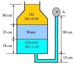
$$P_{A,gage} = (9.81 \text{ m/s}^2)(1000 \text{ kg/m}^3)[0.90(0.80 \text{ m}) + 1(0.35 \text{ m}) - 1.26(0.72 \text{ m})] \left(\frac{1 \text{ kN}}{1000 \text{ kg} \cdot \text{m/s}^2}\right)$$
