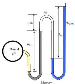
**Discussion** Note that jumping horizontally from one tube to the next and realizing that pressure remains the same in the same fluid simplifies the analysis greatly. Also, it can be shown that the 15-in high air column with a density of 0.075 lbm/ft<sup>3</sup> corresponds to a pressure difference of 0.00065 psi. Therefore, its effect on the pressure difference between the two pipes is negligible.
