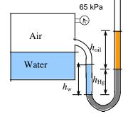
$$\left(\frac{65 \text{ kPa}}{(1000 \text{ kg/m}^3)(9.81 \text{ m/s}^2)}\right) \left(\frac{1000 \text{ kg} \cdot \text{m/s}^2}{1 \text{ kPa.} \cdot \text{m}^2}\right) = 0.72 \times (0.75 \text{ m}) + 13.6 \times h_{\text{Hg}} - 0.3 \text{ m}$$
