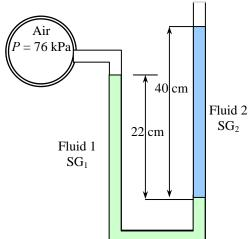
**Discussion** Note that the right fluid column is higher than the left, and this would imply above atmospheric pressure in the pipe for a single-fluid manometer.
