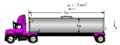
**Assumptions** 1 The acceleration remains constant. 2 Milk is an incompressible substance.
