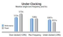
Figure.1 Performance relative to power consumption in single core
