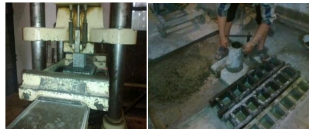
Figure-1 (Compressive Strength Test) (moulds for cubes)
