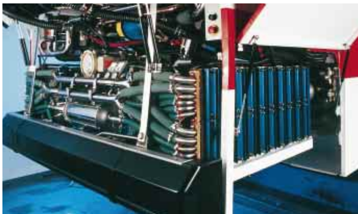
OPERATIONAL BUS built by Ballard Power Systems in Vancouver, B.C., is powered by proton-exchange membrane fuel cells (visible at right). The bus carries compressed hydrogen fuel and emits no pollutants.
