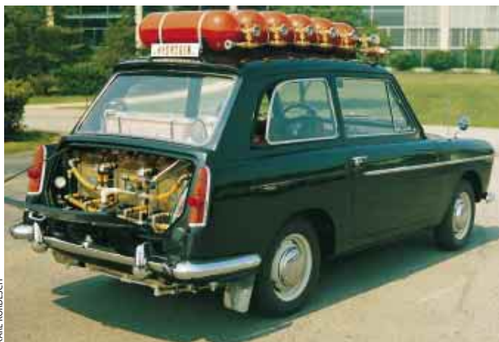
AUSTIN A40 SEDAN was equipped with Union Carbide alkaline fuel cells in 1966 by Karl Kordesch. Though historically important, the vehicle was hardly practical: the cells occupied much of the interior of the passenger compartment. Tanks of compressed hydrogen are visible on the roof.
