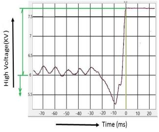
Figure 4: High voltage in KV verses time for 10 KV input for the tested VSD.
