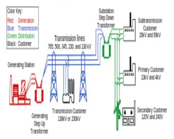
Figure 2: Simplified diagram of AC electricity delivery from generation stations to consumers [12].
