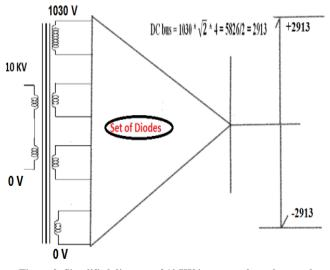
Figure 3: Simplified diagram of 10 KV input supply to the tested VSD.
