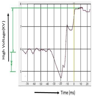
Figure 6: High voltage in KV verses time for 11 KV input for the tested VSD.
