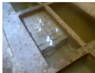
(Curing of cubes)
