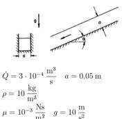
$m^2$   $s^2$ Determine the angle of inclination and the pressure loss per unit length!
