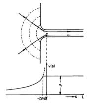
$$\begin{split} \int_{-\infty}^{L} \frac{\partial v}{\partial t} ds &= \int_{-\infty}^{-\frac{D}{\sqrt{8}}} \frac{\partial}{\partial t} \left( \frac{\frac{v_0 \pi D^2}{4}}{2 \pi s^2} \right) ds + \\ &+ \int_{-\frac{D}{\sqrt{8}}}^{L} \frac{\partial v_0}{\partial t} ds = \\ &= \left( \frac{D}{\sqrt{2}} + L \right) \frac{dv_0}{dt} \end{split}$$
