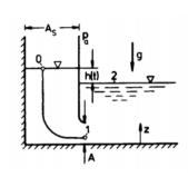
$\begin{array}{rcl} p_a + \rho \ g \ z_0 + \frac{\rho}{2} \ v_0^2 & = & p_1 + \rho \ g \ z_1 \\ & & + \frac{\rho}{2} \ v_1^2 \\ p_1 + \rho \ g \ z_1 & = & p_a + \rho \ g \ z_2 \end{array}$
