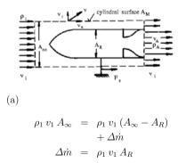
$$\begin{aligned} &-\rho_1 \, v_1^2 \, A_\infty + \rho_1 \, v_1^2 \, (A_\infty - A_R) + \\ &+ \rho_A \, v_A^2 \, A_R + \int_{A_M} \rho_1 \, v_x \, v_r \, dA = F_s \end{aligned}$$
