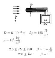
2.5 In order to determine the velocity in a pipe flow the pressure difference  $\Delta p$  is measured. The pressure difference deviates from the dynamic pressure of the undisturbed flow, if there is a large blockage in the pipe.
