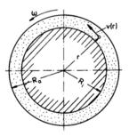
$$\begin{aligned} R_a &= 0.11 \text{ m} \quad R_i = 0.1 \text{ m} \quad L = 0.1 \text{ m} \\ \omega &= 10 \frac{1}{\text{s}} \quad M_z = 7.246 \ 10^{-3} \text{ Nm} \end{aligned}$$
