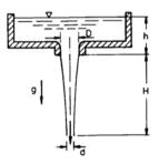
h = 0.1 m H = 1.5 m D = 0.1 mWhat is the diameter d of the water stream at the position H below the opening?
