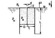
$$\begin{array}{rcl} p_1 + \rho_B \; g \; z_1 + \frac{\rho_B}{2} \; v_1^2 &=& p_a + \frac{\rho_B}{2} \; v_2^2 \\ p_a &=& p_1 + \rho_w \; g \; z_1 \\ v_1^2 \; \ll \; v_2^2 \\ v_2 \; d^2 &=& v_1 \; D^2 \\ &=& \frac{dz_1}{dt} \; D^2 \end{array}$$
