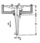
$$\begin{split} \rho \, g \, (h+H) &= \rho \, g \, H + \frac{\rho}{2} \, v_1^2 \\ &= \frac{\rho}{2} \, v_2^2 \\ v_1 \, D^2 &= v_2 \, d^2 \\ d &= D \, \sqrt[4]{\frac{h}{h+H}} &= 0.05 \; \mathrm{m} \end{split}$$
