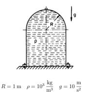
Determine the force in the screws under the assumption that the weight of the container can be neglected!
