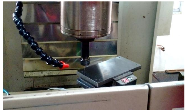
Fig 8 Workpiece mounted on CNC Vertical Milling Machine
