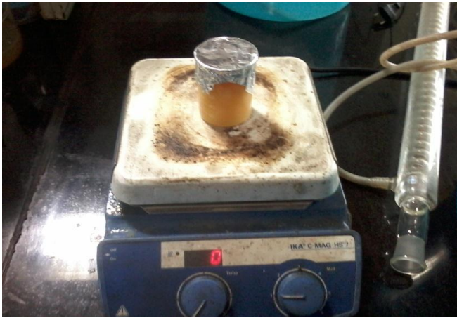
Fig 7 Nanofluid mixing using magnetic stirrer
