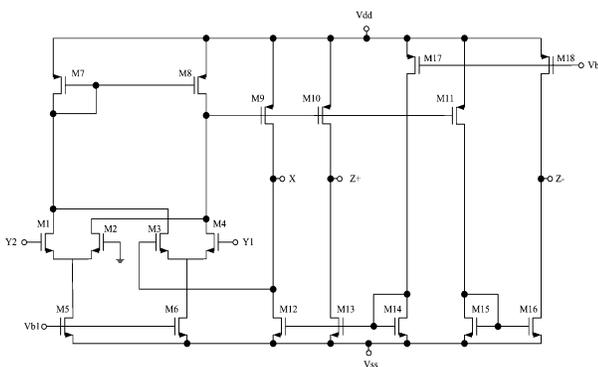
**Figure 2.** CMOS implementation of the DVCC.
