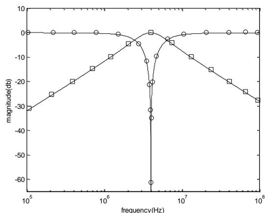
**Figure 4.** CM and normalized TIM amplitude-frequency responses with notch and bandpass signals of the proposed biquadratic filter (○, simulated notch; □, simulated bandpass; and —, theoretical curve).
