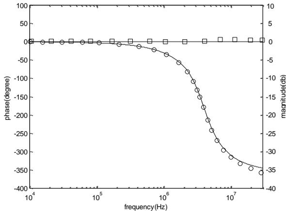
**Figure 5. Phase-frequency and amplitude-frequency responses with CM and normalized TIM allpass signals of the proposed biquadratic filter (○, simulated phase; □, simulated amplitude; and —, theoretical curve).**
