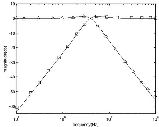
**Figure 3.** CM and normalized TIM amplitude-frequency responses with highpass and lowpass signals of the proposed biquadratic filter (□, simulated highpass; Δ, simulated lowpass; and —, theoretical curve).
