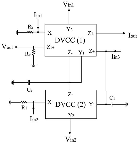
**Figure 1. Proposed mixed-mode biquadratic filter structure.**
