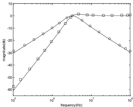
**Figure 6. VM and normalized TAM amplitude-frequency responses with highpass and bandpass signals of the proposed biquadratic filter (□, simulated highpass; ○, simulated bandpass; and —, theoretical curve).**
