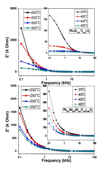
Fig.-1: Temperature-frequency dependence of Z' of PZT and PGZT ceramics
