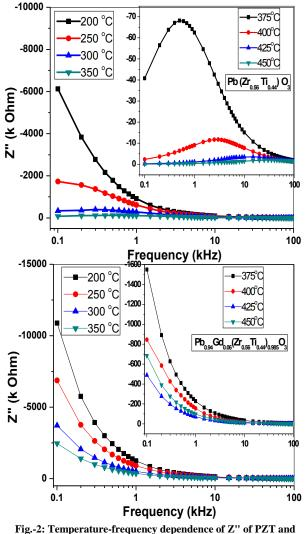
Fig.-2: Temperature-frequency dependence of Z" of PZT and PGZT ceramics
