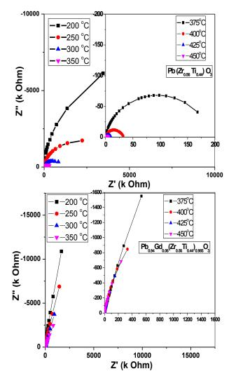
Fig.-3: Temperature-frequency dependence of Z'' of PZT and PGZT ceramics
