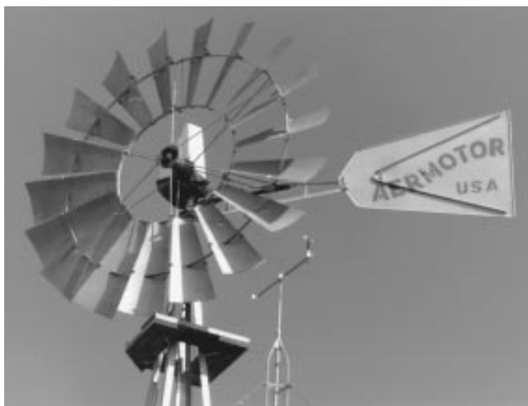
FIGURE 7.7.1 The multivane American windmill Photograph by Paul Gipe. (Adapted from Wind Power for Home & Business , Chelsea Green Publishing, 1993).
